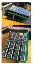
Stack the boards, add "on/off" and "prgm/run" switches, Make a simple wood box, it's done!
